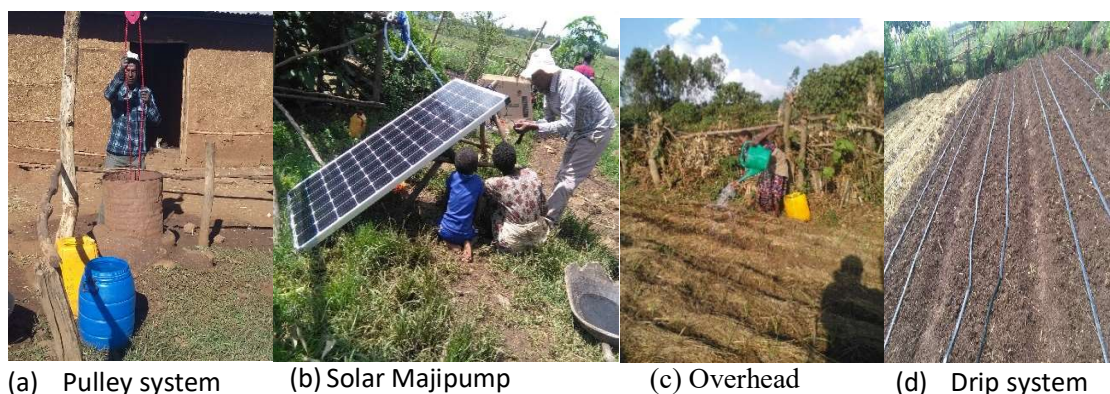
Figure 5- 4: Water lifting and irrigation technologies used during the experimental period (2016-2019), modified pulley water lifting system (a), solar-driven Majipump water lifting system (b), overhead water application system using watering-can (c), and drip irrigation system (d).
