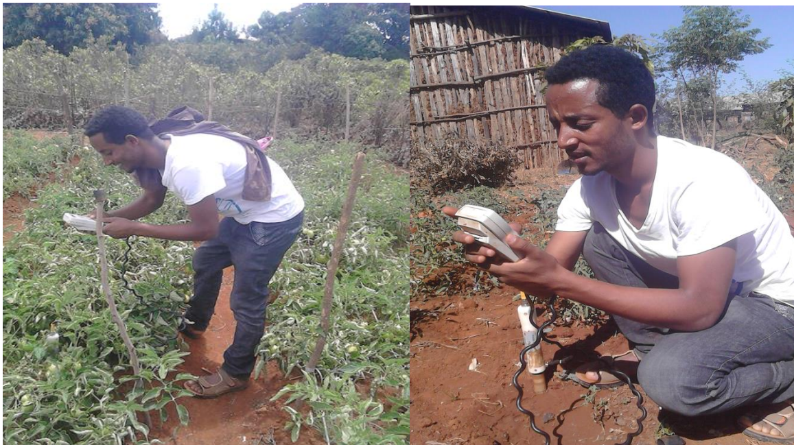
Figure 3-5: Soil moisture measurements using the profiler tube.
