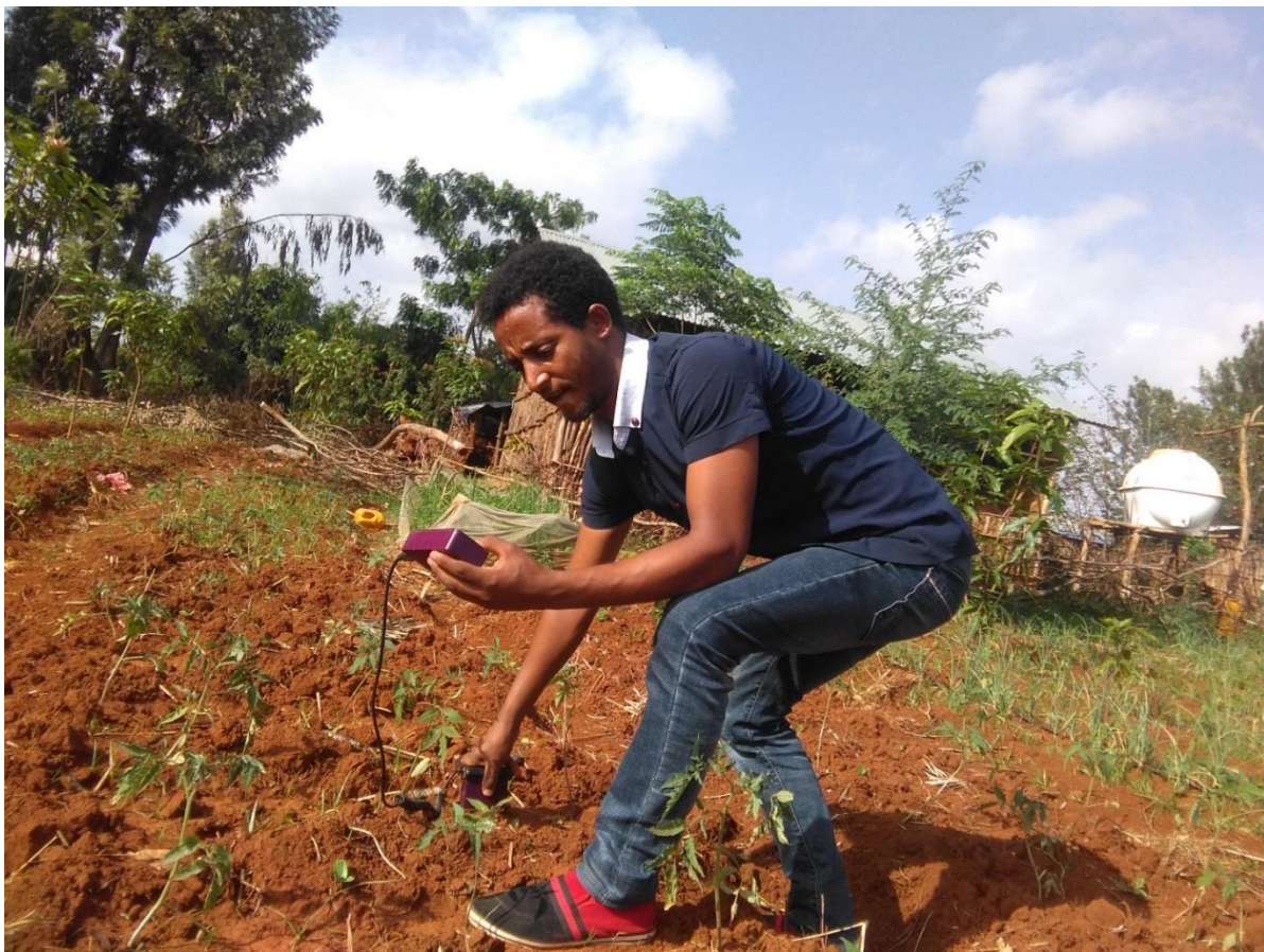
TDR reading at the initial stage during early 15 days after planting of tomato.
