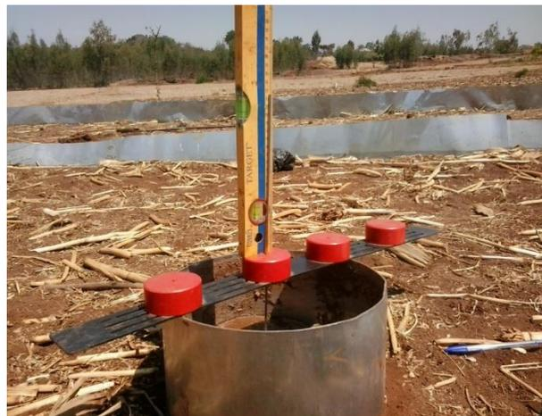
**Picture S1: Measuring pre treatment left and post treatment right steady state infiltration rate**
