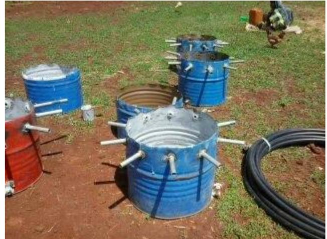
**Picture S6: Tank for runoff collection (runoff barrel)**
