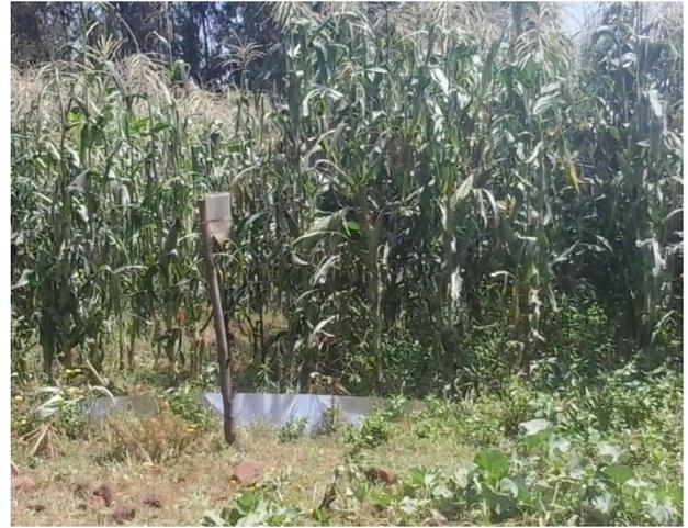
**Figure 3.4: Runoff barrels (left) and manual rain gauge (right) installed to collect surface runoff and daily rainfall respectively**
