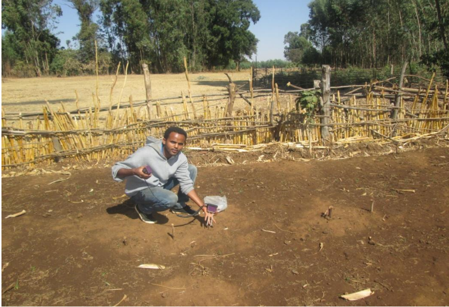
Measuring initial soil moisture reading by TDR
