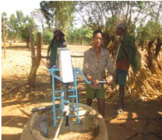
Figure3-3: Rope & Washer (left) and the improved Pulley with tanker and delivery hose (right).
