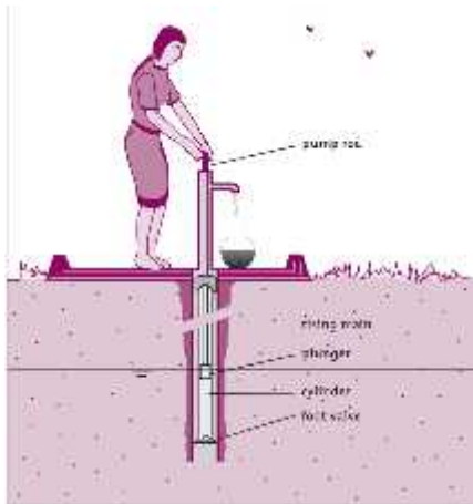
Fig 2.3.5 Direct action hand pump (Source: Arlosoroff et al, .1987; Morgan et al., 1990; Reynolds, 1992).
