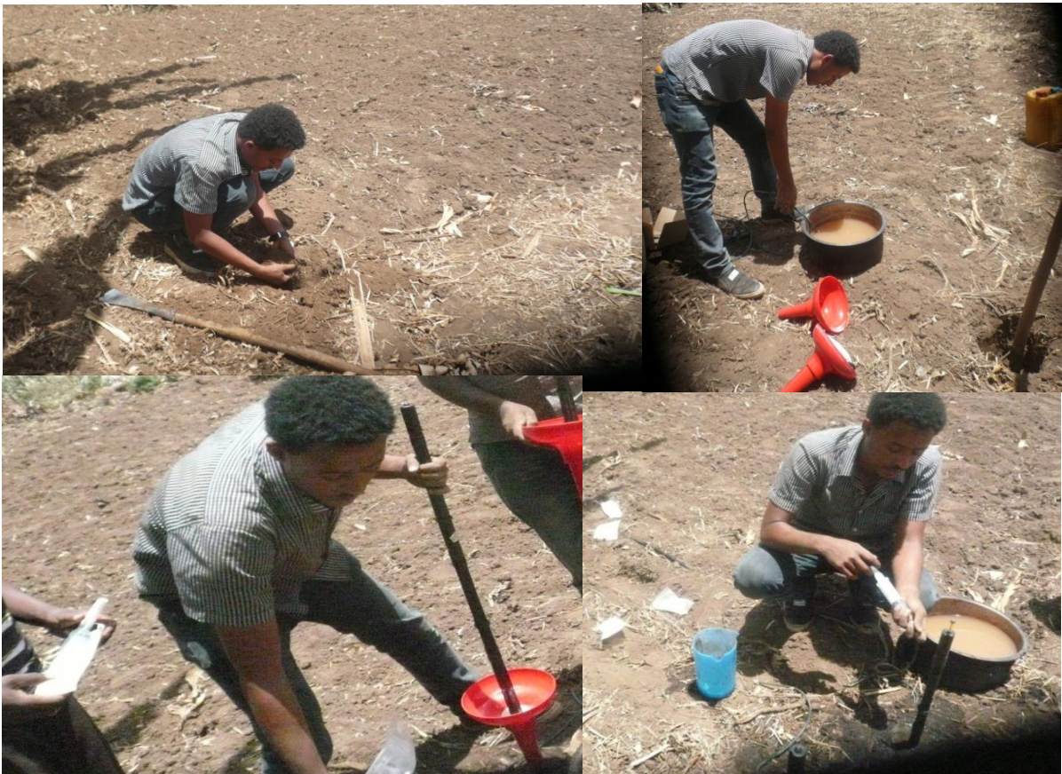
Figure 3.5: Wetting Front Detector Installation
