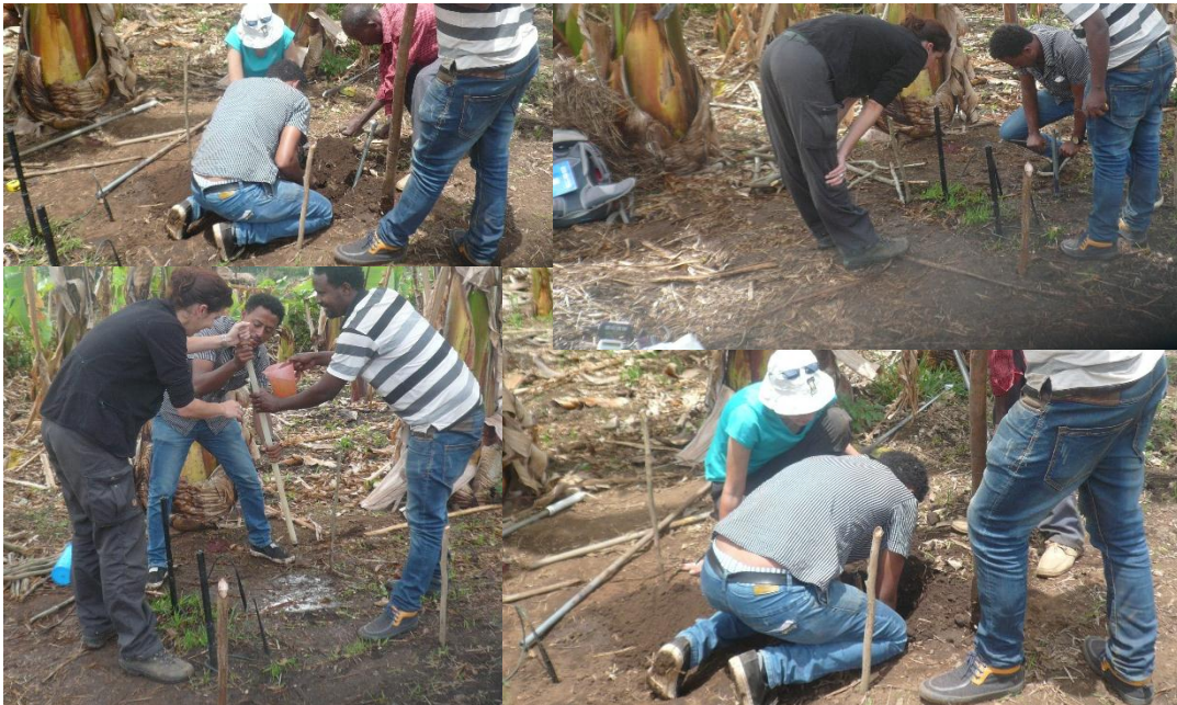
Figure 3. 6: Soil moisture profiler installation
