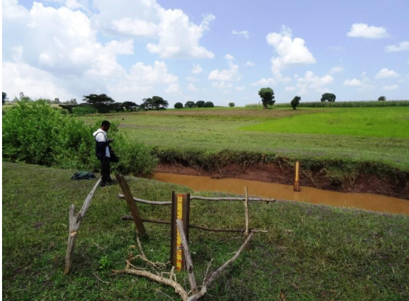
Figure 3-4 Staff gauge which was installed at the total watershed outlet
