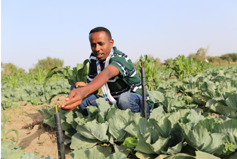
Photo: Development Agent in Ethiopia demonstrates the wetting front detector. Photo Credit: Apollo Habtamu
