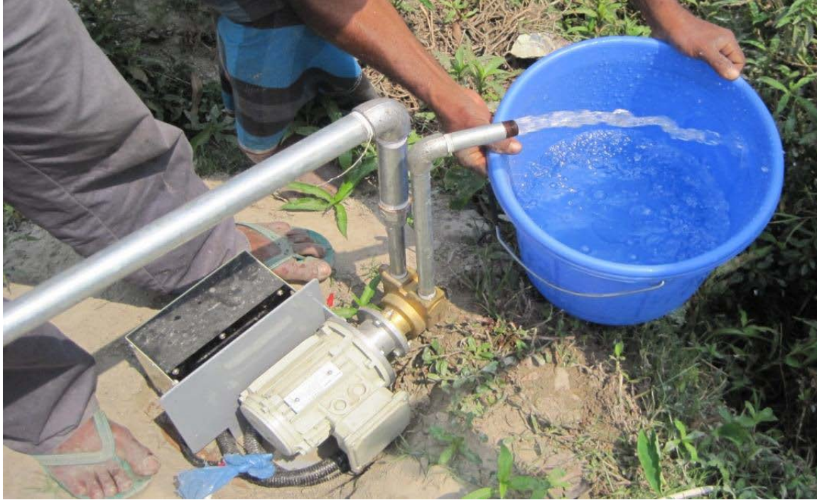
Prototype of a small-scale solar pump developed by BUAS (Rangpur, Bangladesh). (Source: Imoberdorf, K. MSc thesis, 2012)
