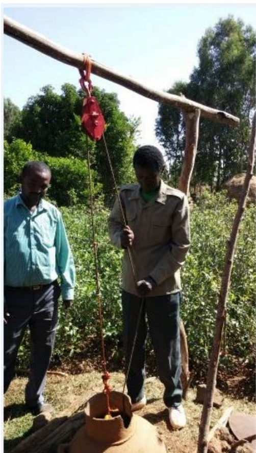
Pulley/Bucket system (Bahir Dar, Ethiopia)
