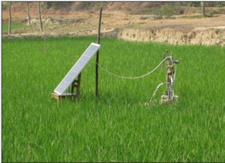
Solar pump in rice field in Rangpur, Bangladesh. (Source: Imoberdorf, K. MSc thesis, 2012)
