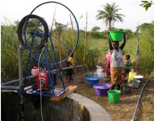
Gasoline-motor-powered rope-and-washer pump
