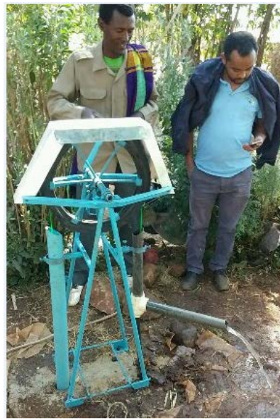
Hand-operated rope-and-washer pump
