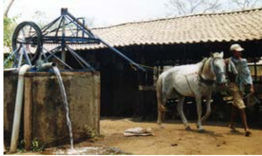
Rope-and-washer pump operated by horse
