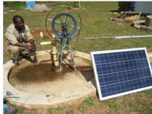
Solar-powered rope-and-washer pump
