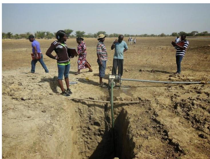
*Motorized pump and shallow well*
