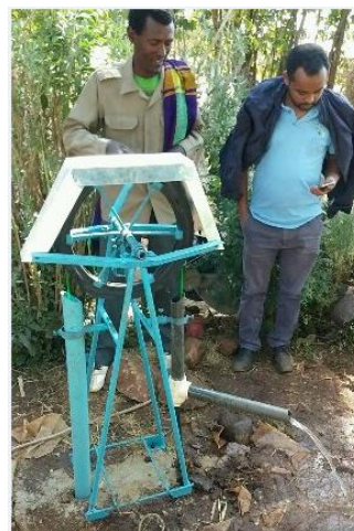
Figure 7: Hand-operated rope-and-washer pump
