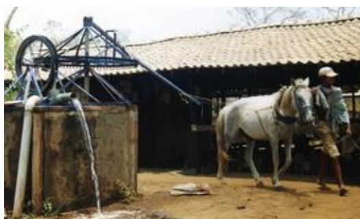
Figure 8: Rope-and-washer pump operated by horse
