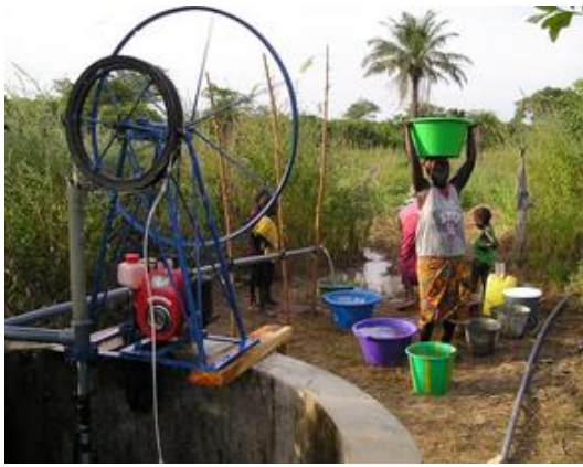
Figure 9: Gasoline-motor-powered rope-and-washer pump
